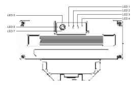
①LED1, LED2, LED3, LED4 are white lights and show the battery SOC and lifespan ②LED5, LED6, LED7 are red, orange, and white lights respectively and show the status of the battery's health
